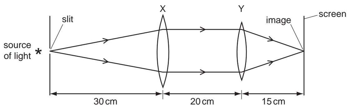
What are the correct values for the focal lengths of X and of Y?
