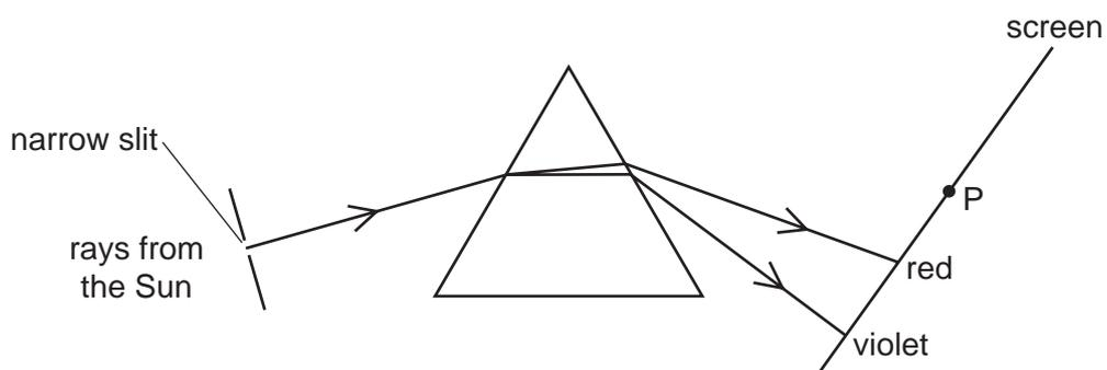
A thermometer placed at P shows a large temperature rise.
